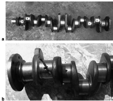
(a) General view of the failed crankshaft and (b) close-up view of fracture location.
